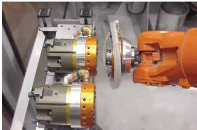
Quick change grippers on a storage rack for automatic change between parts.
