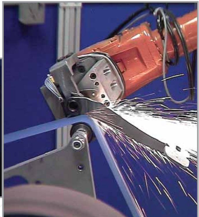
Belt Head for Small Radius Polishing
