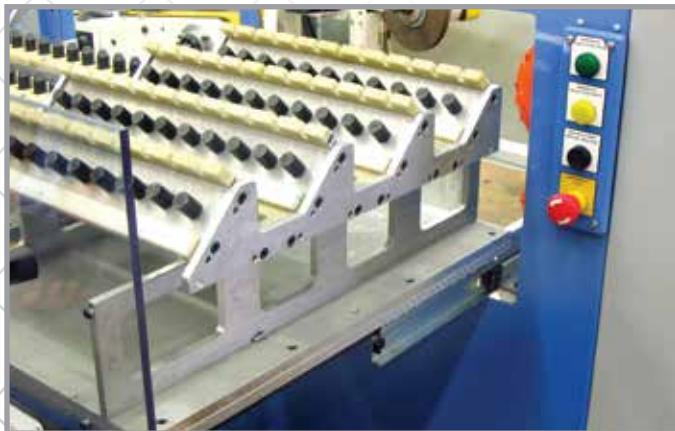
Multiple Part, Dual Slide-in Drawer (Load one while other is running for continuous operation.)
