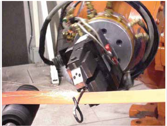
Formed gripper for small parts.
