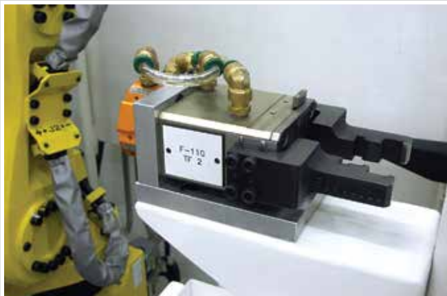
Single rack quick change gripper.
